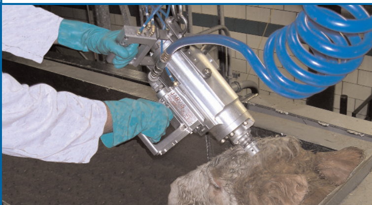
Non-penetrating stunner used with monorail restrainer.
